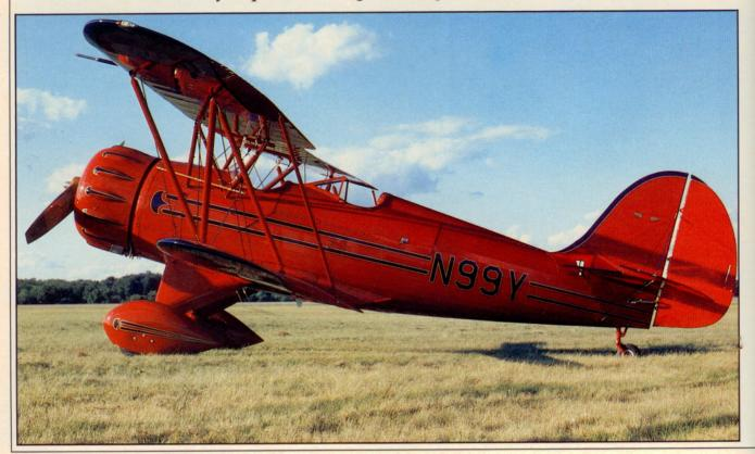
powered. They also featured refinements such as wings with a 50-percent stagger for better visibility and, on later versions, the Clark Y airfoil, which became the standard for light aircraft designs in the 1930s because of its high coefficient of lift and relatively gentle stall characteristics.
